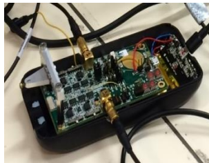
Portable 8 channel amplifier made in Zw ©2015 - RAM Group DE GmbH Temperature, pH, DC and high- frequency AC recording
